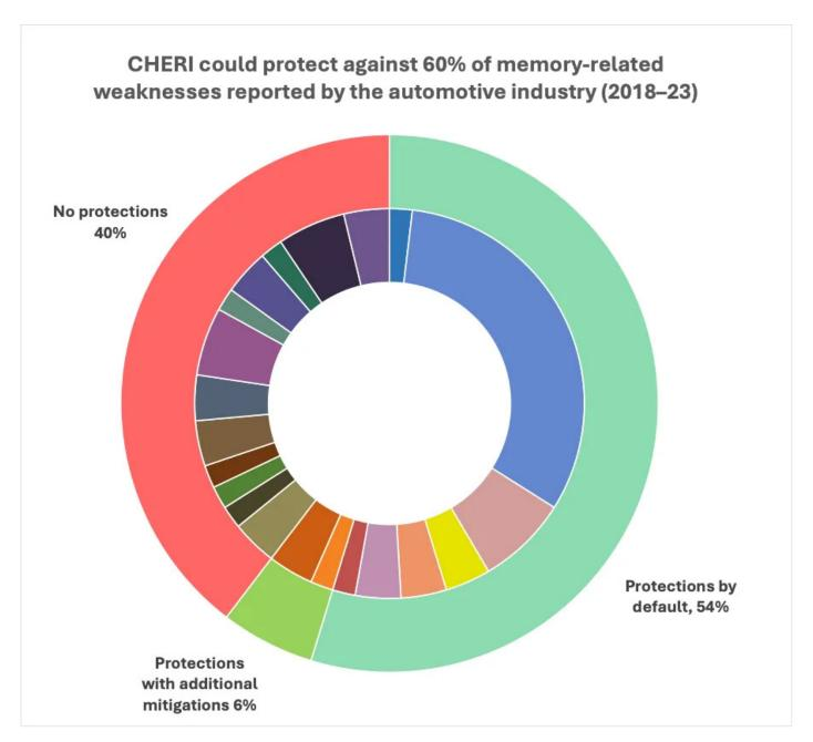
CHERI would protect against the majority of memory-related weaknesses, including the frequently observed out-of-bounds write, straight out of the box. With the implementation of additional mitigations, the total number of weaknesses prevented could hit 60%.
